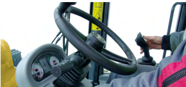
Electrical proportional adjustment of the hydraulic performance of the 3rd circuit.
