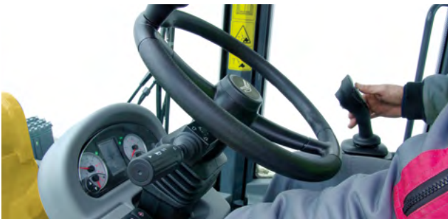
Electrical proportional adjustment of the hydraulic performance of the 3rd circuit.
