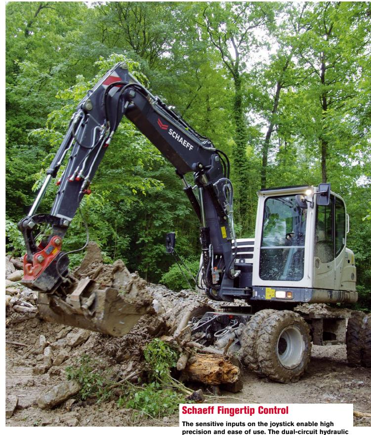
system with load independent flow sharing (LUDV) allows simultaneous, independent work movements. Economic load sensing technology ensures accurate volume control, hence saving fuel.
